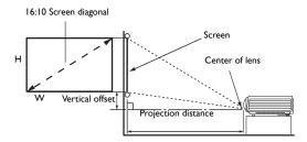
The screen aspect ratio is 16:10 and the projected picture is 16:10
