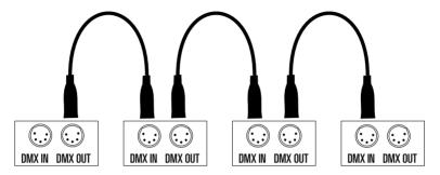
joined (apart from end-to-end) or split. Using a 2-to-1 splitter or similar will prevent the system working.
