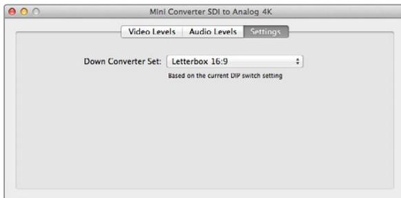
Adjust down conversion settings using Blackmagic Converter Utility.
