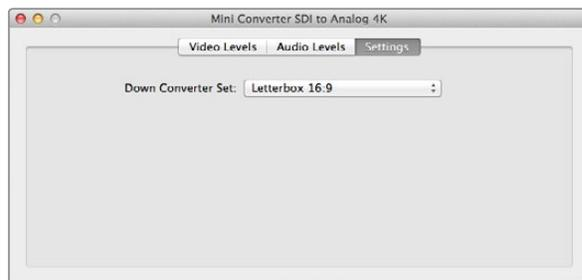
Adjust down conversion settings using Blackmagic Converter Utility.
