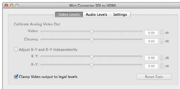
The Clamp Video output to legal levels setting is checked by default. This setting ensures your analog output is a true representation of the SDI input. Adjusting video levels may result in illegal colors.
