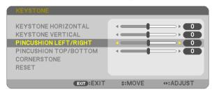
3. Press the ◀ or ▶ button to correct distortion.
