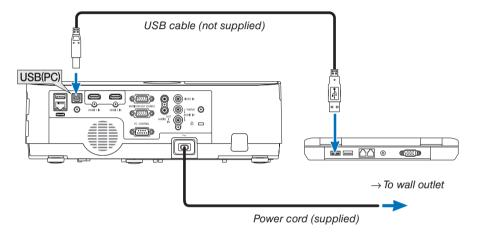
The message "The projector is in standby mode. Connect it?" will be displayed on the computer screen.
