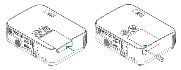
This completes the lamp replacement. Go on to the filter replacement.
