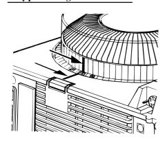
Projectors are often installed on racks where tray installation may be difficult and only possible from the rear of the projector. In this case the tray positioning index mark (27) on the back of the projector is very helpful: The tray is properly set when the index mark aligns with the mark placed on the tray (at slide no. 20 of the 80 slide tray and at slide no. 35 on the 140 slide tray).
