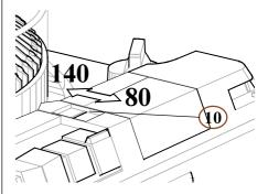
Round trays for both 80 slides and 140 slides can be used. The tray setting switch (10) is set in the factory to accommodate the 80 tray. By using a small screwdriver, the switch can be brought into the 140 position.
