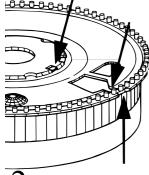
• Check that the baseplate of the slide tray is locked into zero-position and cannot be rotated.
