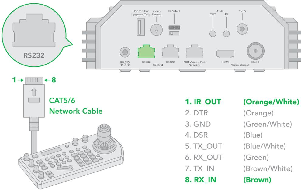
8. Make an RS232 Daisy Chain multiple camera connection with a standard RS232 serial port controller:
