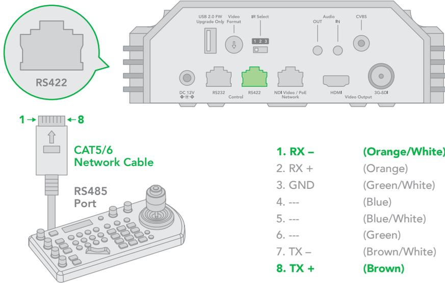
10. Making connections for multiple cameras using RS485 standard serial port controller.
