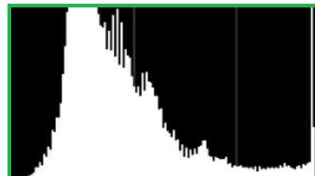
**Waveform:** The Waveform scope shows the distribution of luminance in the image as a waveform that ranges from zero at the lower horizontal line, to 100 % intensity at the upper horizontal line. The left to right position of the values match their position in the image.
