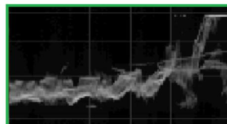
**RGB Parade:** The RGB Parade shows the intensity of Red, Green and Blue in the image as separate waveforms that range from zero at the lower horizontal line, to 100 % intensity at the upper horizontal line. For each waveform, the left to right position of the values match their position in the image.
