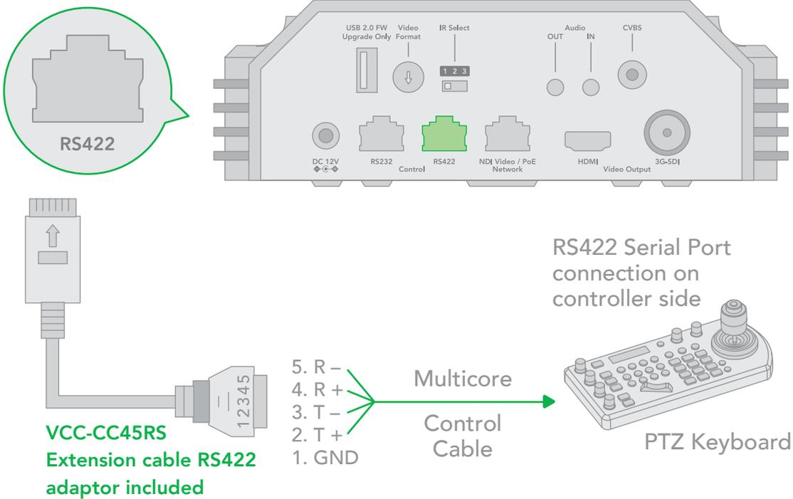
6. You can use a CAT5/6 T-568B cable to make an RS422 direct connection between the camera and the controller by following the pin definition below.
