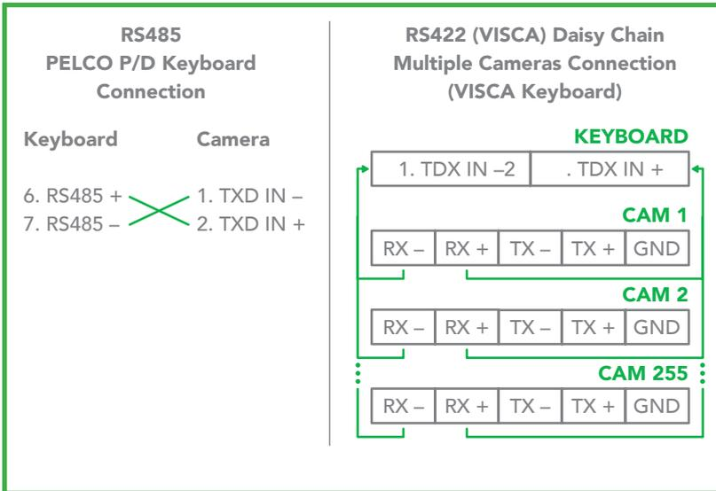
8. Use the included RJ45 to RS422 cable with a Phoenix connector adaptor to make an RS485 connection for your control device.
