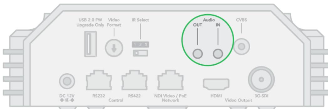
Analog 3.5mm audio In/Out ports. The Audio Out will output any audio that is captured on the Audio In port. Audio format is stereo, unbalanced line level.
